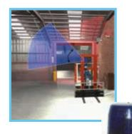
Each forklift is fitted with a transmitter (Beacon) that sweeps a coded infrared (No RF) beam around the forklift and transmits downwards (-20°) and upwards (+60°). Note: This beam is invisible
