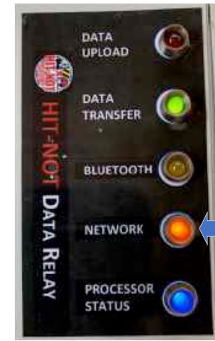
Must have solid Orange light on the Network before the REM Relay will work.
